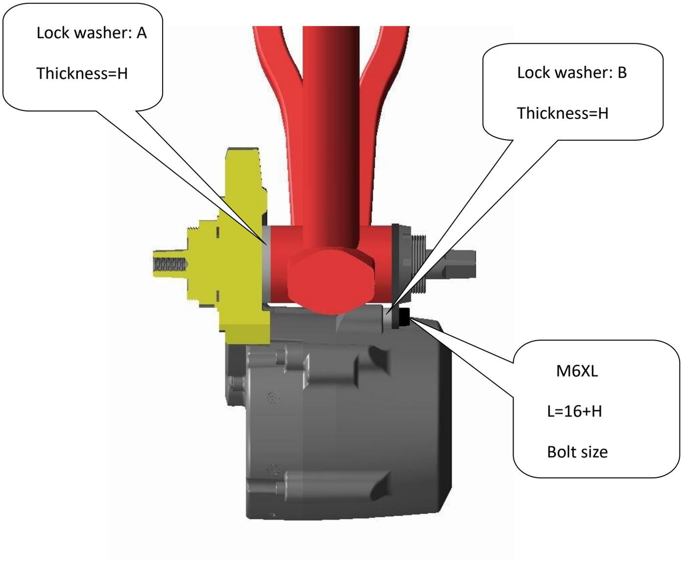
Note: the thickness H of lock washer A and lock washer B must be equal
